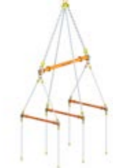
One Over Three 6 POINTS OF LIFT
