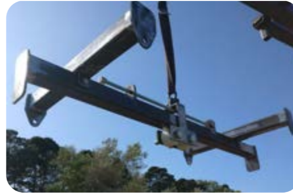
H-Frame with adjustability for offset CoG
