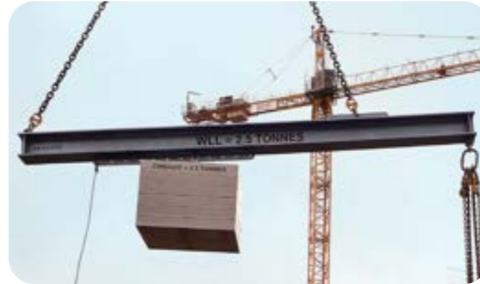
Counterweight Lifting Beam – WLL 2.5 tonne
