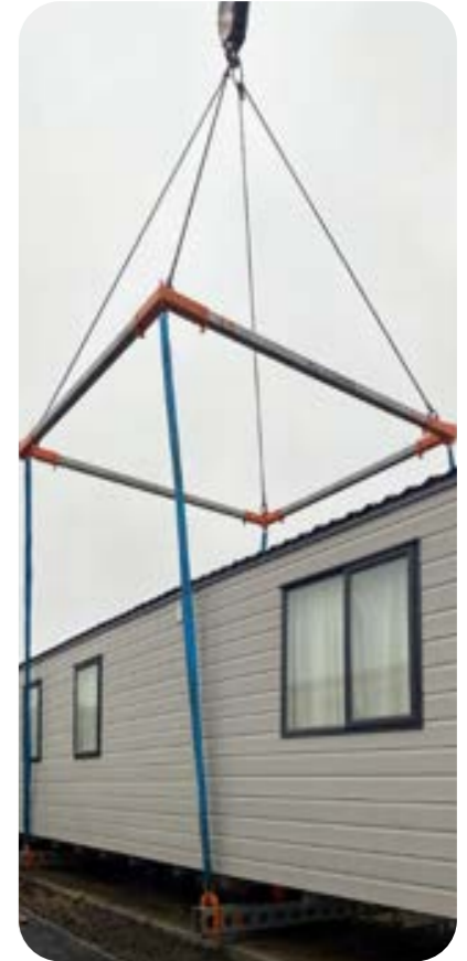
Spreader Frame with removable struts
