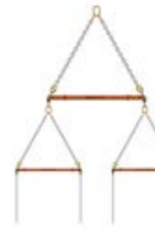
One Over Two Inline 4 POINTS OF LIFT
