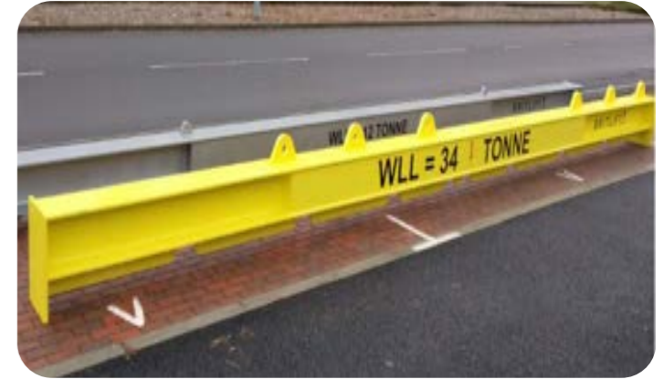
Module lifting system with 10m adjustable lifting beam
