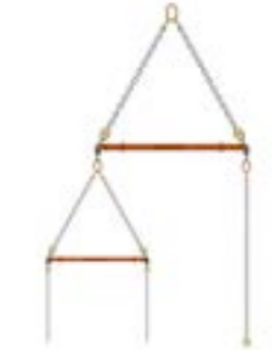
One Over One Inline 3 POINTS OF LIFT
